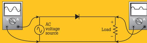
Figure 5. Half-wave rectifier circuit.
