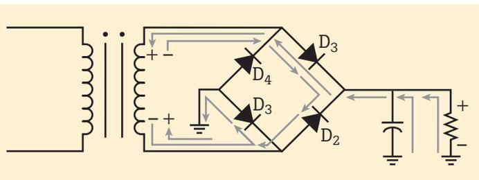
Figure 4. Bridge rectifier with multiple diode failures.
