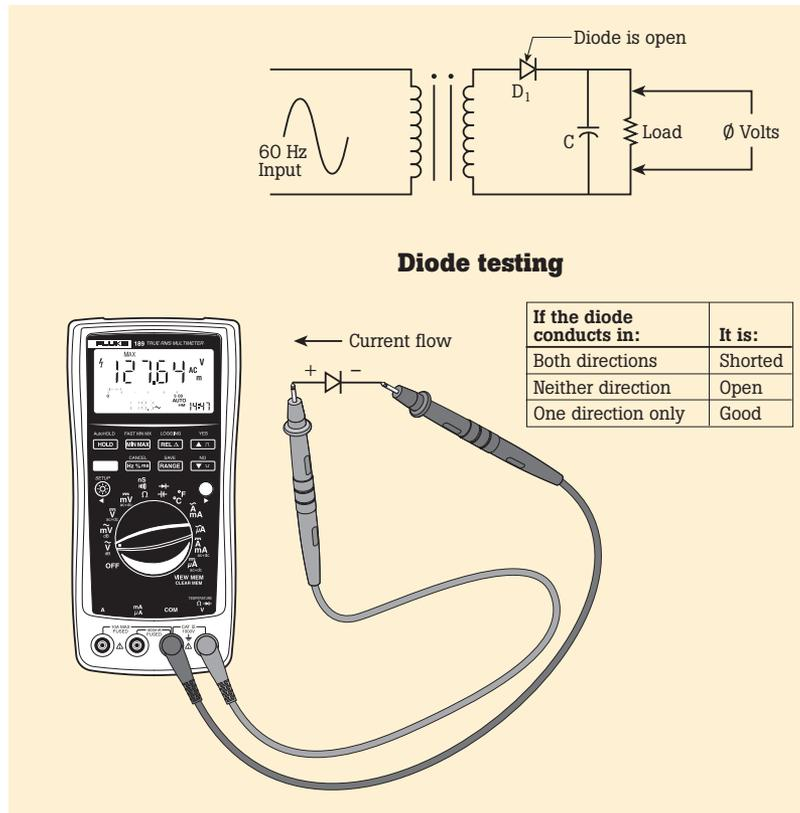
Figure 1. Half-wave rectifier with failed diode.
